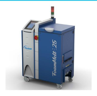
The Standard FoamMelt FIT25 melter uses proven Nordson Automatic Density Control technology to achieve the required foam density reduction. It features a Manual Density Controller that employs a density sensor to regulate gas injection to achieve and maintain the desired foam density reduction.
